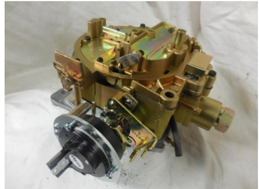
You will need to provide the electric choke coil with **+12V off a keyed ignition source.**
