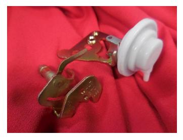
11) Now install the Buick choke arm into your Chevrolet choke bracket, tapping it firmly in place, pressfit.
