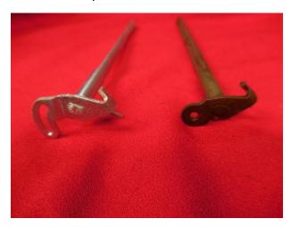
4) First remove the four screws holding the air flaps on the shaft, and set the flaps aside. (You may need to remove the air horn and grind the staked ends off them, but not in all cases.)
