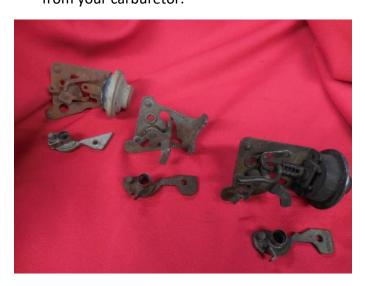
3) There were two distinct styles of secondary air flap shaft end. If your carb has the shaft on the left below, skip to #8. If your carb has the shaft on the right below, it must be swapped out for the style on the left...Acquire the correct style shaft and continue to #4.
