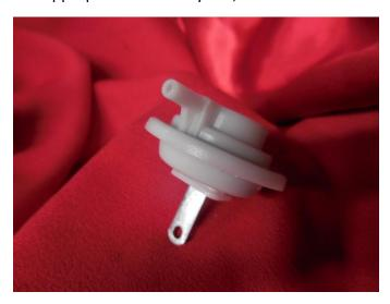
Two links work equally well. One hooks into the pulloff, and the other inserts thru and is held in place by a clip. Quadrajetparts.com #3051
