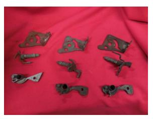
10) Acquire a Buick choke bracket and do the same. Compatible 1968-1974 Buick choke arm numbers are 38728, 38729, 50728, 33165, 37303, 37257.
