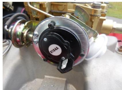
21) Hold the throttle open a little and rotate the electric choke coil Counter Clockwise until the primary choke flap is fully closed on top of the carb. Tighten the three #6-32x1/4 screws to lock the electric choke coil in place.
